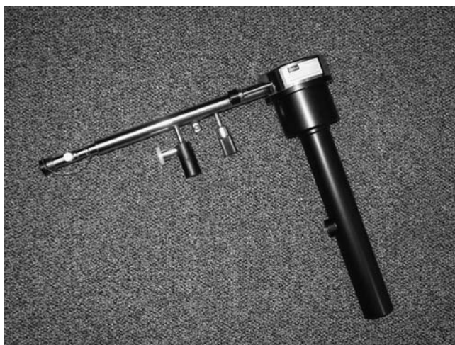
Fig. 9.4 Bruker/Oxford CF935 continuous flow cryostat for liquid He and liquid N 2 operation
